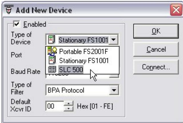
When SLC 500 device is chosen, button Connect will change to button Advanced.
