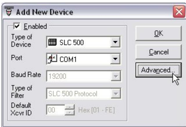
**Advanced** button will take you to the Advanced PLC Properties Window where you can add commands to be sent to all readers when the PLC state changes from Start to Stop.
